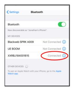
5. If the printer SN# does not show up in your Bluetooth settings screen, Hold in the blue paper feed button on the far right of the printer until the BT icon starts flashing on the printer screen. Once it starts flashing, it should also come up on the device (phone) screen. Select "Pair" on the prompt then immediately press the yellow check mark button on the printer.
