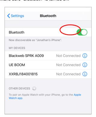
4. On your phone, tap on the Bluetooth device with the same number. (SN# usually start with XXRB...) The printer should show connected.
